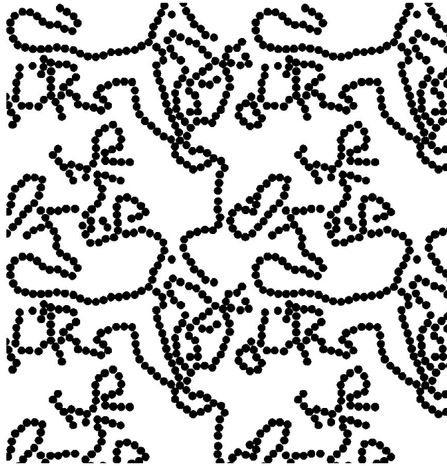
FIGURE 1.3. Dipolar network — A simulation of a self-assembling network (2D) composed of dipolar hard spheres by Davis et al. [93].
